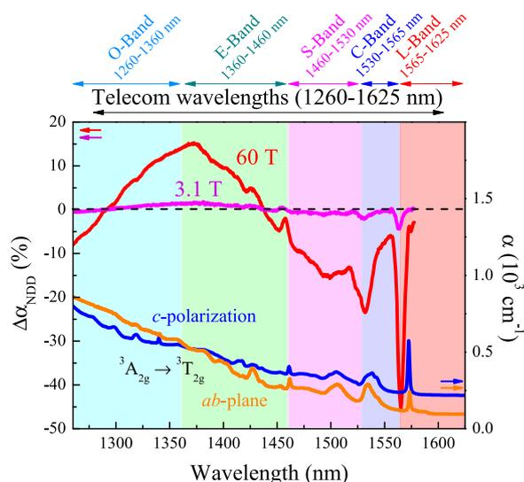
**Fig. 4 Nonreciprocity at telecom wavelengths.** Close-up view of nonreciprocal directional dichroism in  $\text{Ni}_3\text{TeO}_6$  on a percentage basis as a function of wavelength in the toroidal configuration at 4.0 K.  $\Delta\alpha_{\text{NDD}}$  is shown at 3.1 and 60 T. The absolute absorption spectrum is included for comparison. Various commercial telecom windows are summarized on the upper axis. The U-band (1625–1675 nm) is not shown.
