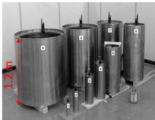
Fig. 1. Photograph of 9 magnet coils of the 60TCW magnet.
