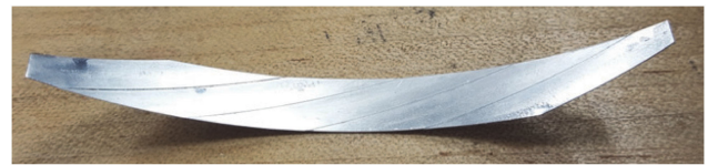
Fig. 4. Crossover laminate with 5 REBCO conductors soldered to copper foil.
