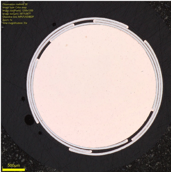
Figure 8. Cross section of straight CO CORC® wire.
