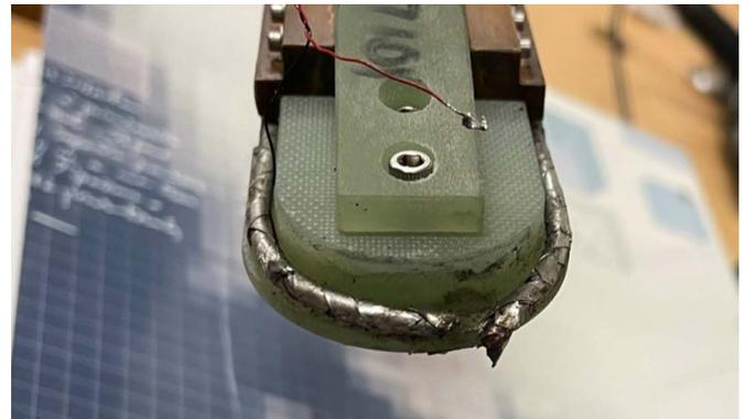
**Figure 12.** Photograph of 2.52 mm diameter STAR<sup>®</sup> wire fabricated with 12 strands of tape, showing burn-out after testing at currents of over 2,500 A at 4.2 K, 30 T.
