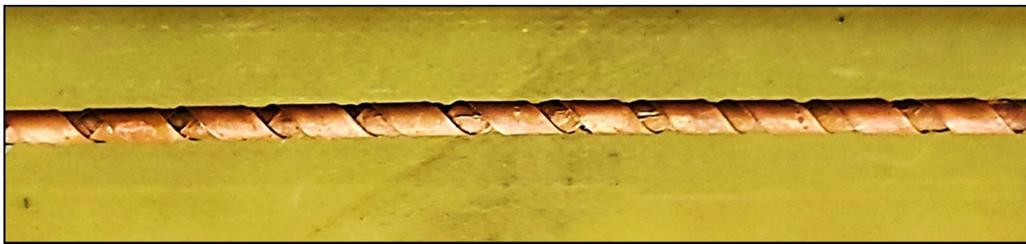
**Figure 5.** Photograph of a 1.51 mm diameter round REBCO wire made with four  $\sim 2$  mm wide tape strands. The tape strands were made with high-performance advanced MOCVD REBCO tape consisting of 4  $\mu\text{m}$  thick film,  $(\text{Ba} + \text{Zr})/\text{Cu} > 0.72$ .
