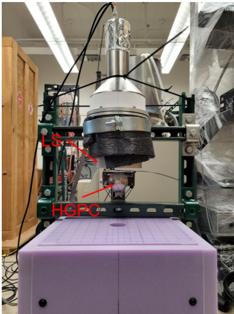
Figure 15. The setup for measuring SbBe neutron tagging with EJ-301 LS.
