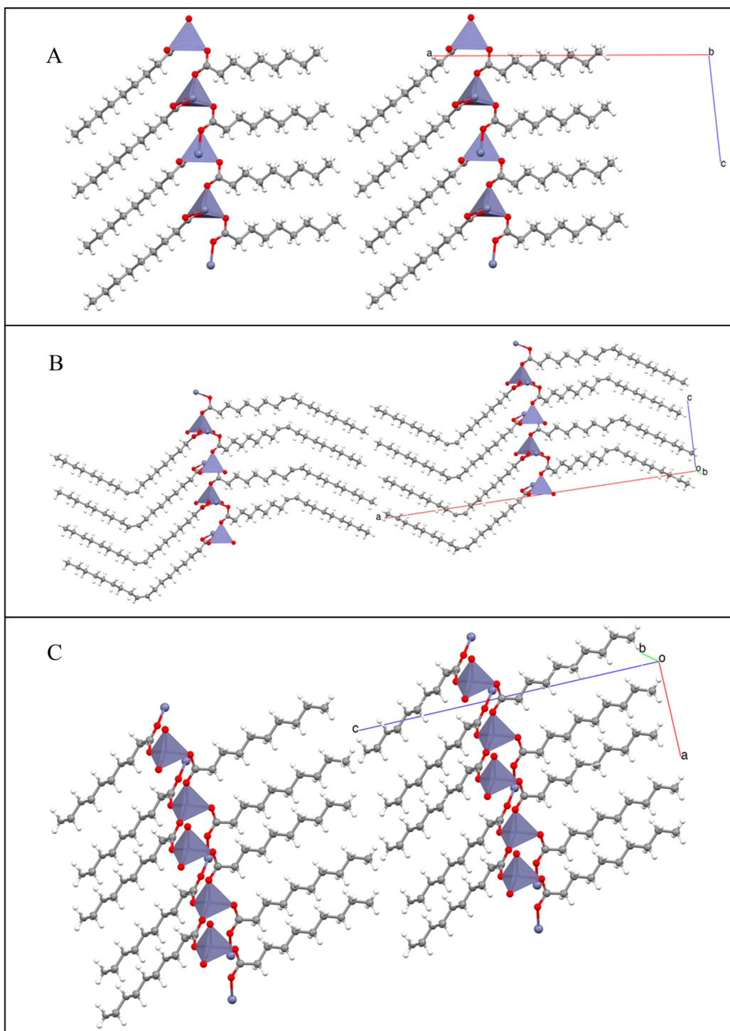
**Fig. 2** Structures of group I represented by ZnC9 (A) and ZnZ-C18 (B), and group II represented via ZnC10 (C) highlighting the arrangement of tetrahedron about the zinc in each crystal type. Hydrogens have been removed for visual clarity.
