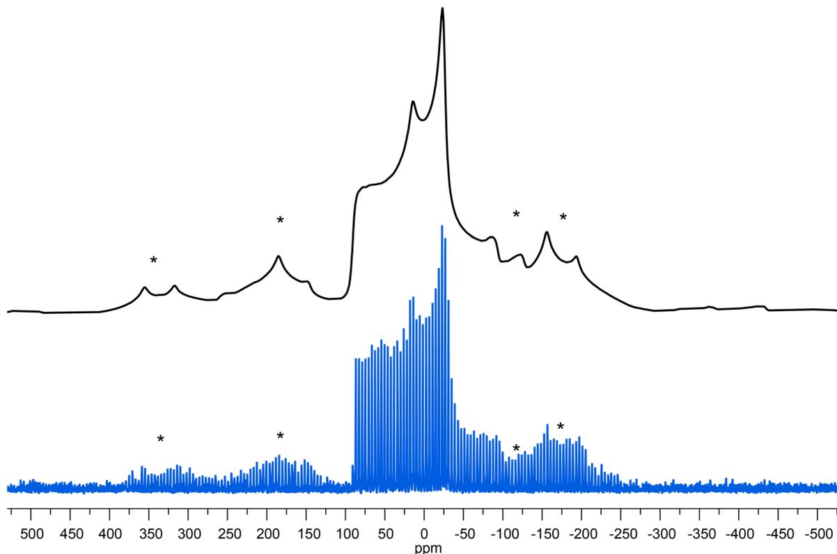
**Fig. 8**  $^{67}\text{Zn}$  spectra for ZnPIV. (Top, Black) Ssnake fitting parameters visualized in TopSpin; (Bottom, Blue) WURST-QCPMG spectrum at 16 000 Hz MAS. Sideband regions denoted with asterisks.  $B_0$  35.2 T.
