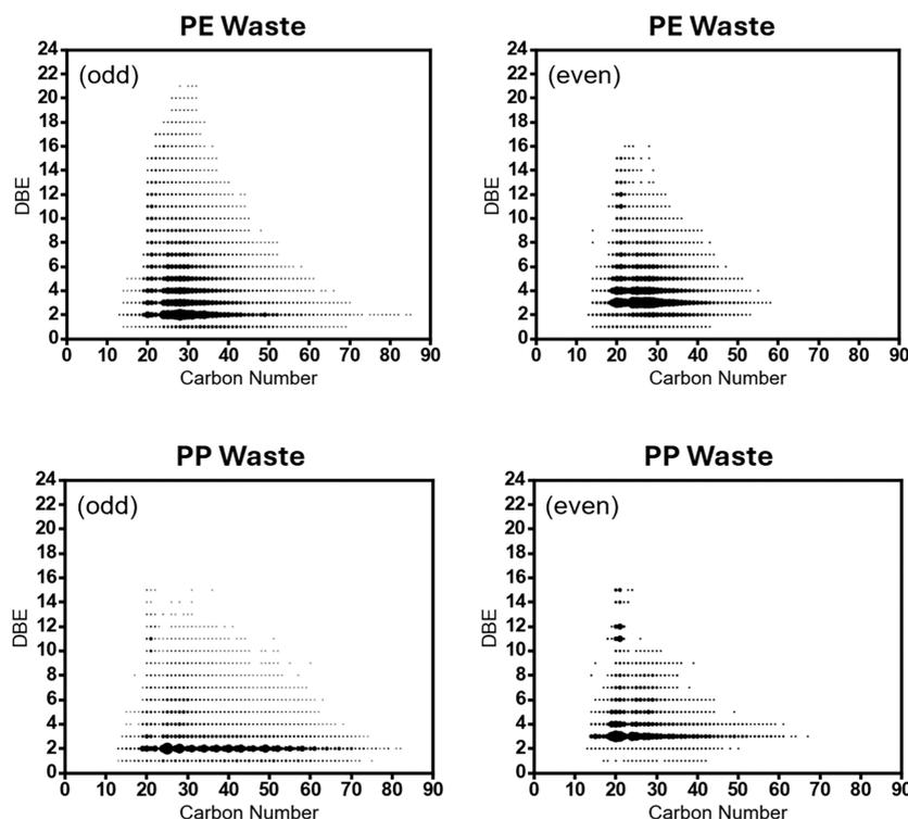
**Figure 3.** Carbon number vs DBE plot for the hydrocarbons in PE (top) and PP (bottom) waste pyrolysis oil with odd-electron ions (left) and even-electron ions (right) for (+)APPI FT-ICR MS. The area of the dots is proportional to the relative abundance of the respective molecular formula.
