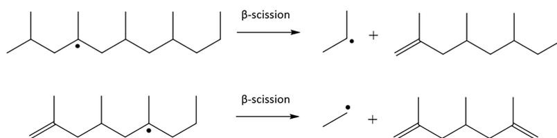
**Figure 6.** Illustrative reaction mechanism for the formation of iso-olefins and diolefins in PP pyrolysis.
