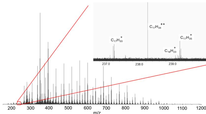
**Figure 1.** Raw mass spectrum of the PE waste pyrolysis oil obtained by (+)APPI FT-ICR MS and enlargement of 237–239 nominal mass.
