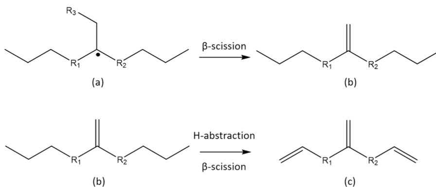
**Figure 4.** Illustrative reaction mechanism for the formation of triolefins during thermal pyrolysis of polyolefins.
