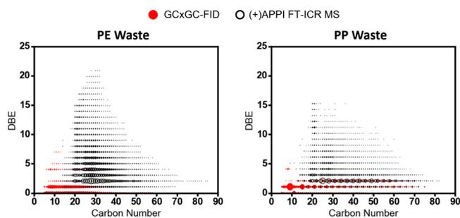
**Figure 8.** Carbon number vs DBE plot for the PE waste pyrolysis oil (left) and PP waste pyrolysis oil (right) for GC  $\times$  GC-FID (red) and (+)APPI FT-ICR MS (black). The area of the dots is proportional to the abundance of the respective molecular formula for FT-ICR MS and GC  $\times$  GC-FID.
