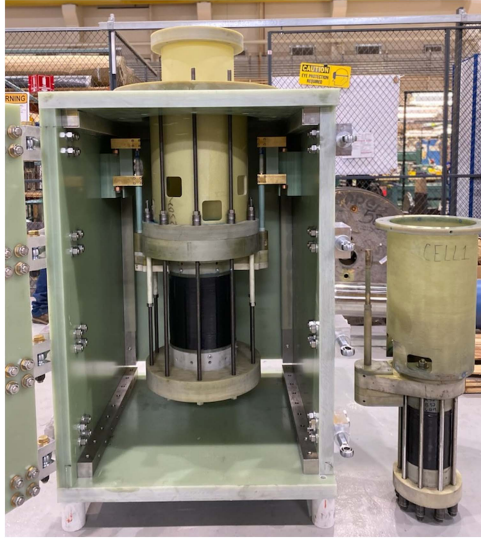
Fig. 8. Picture of 85T duplex magnet and its power delivery fixture mounted inside a strong G-10 blast-box.
