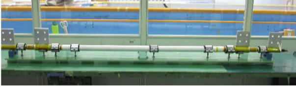
Fig. 1. Measured sample cable. The silver part in the central area is the outer shield conductor, and two copper plates at both the ends are attached to the inner core conductor.
