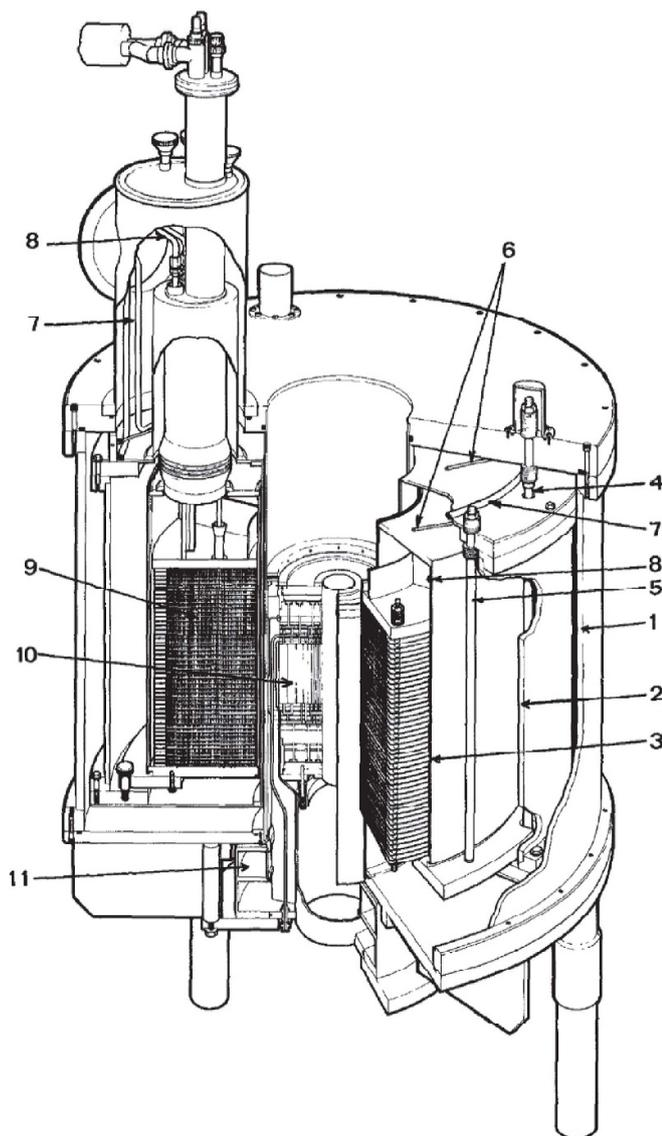
**Figure 2.** Isometric drawing with partial vertical section of the first hybrid magnet to be put into service [11]. Components (1) Outer vacuum vessel (2) Radiation Shield (3) Liquid helium can. (4) Support tube–outer case to radiation shield. (5) Support tube–radiation shield to helium can. (6) Radial support rods (7) 50 K refrigeration lines. (8) 20 K refrigeration lines (9) Superconducting magnet. (10) Water-cooled magnet. (11) Cooling water manifold and current terminals.
