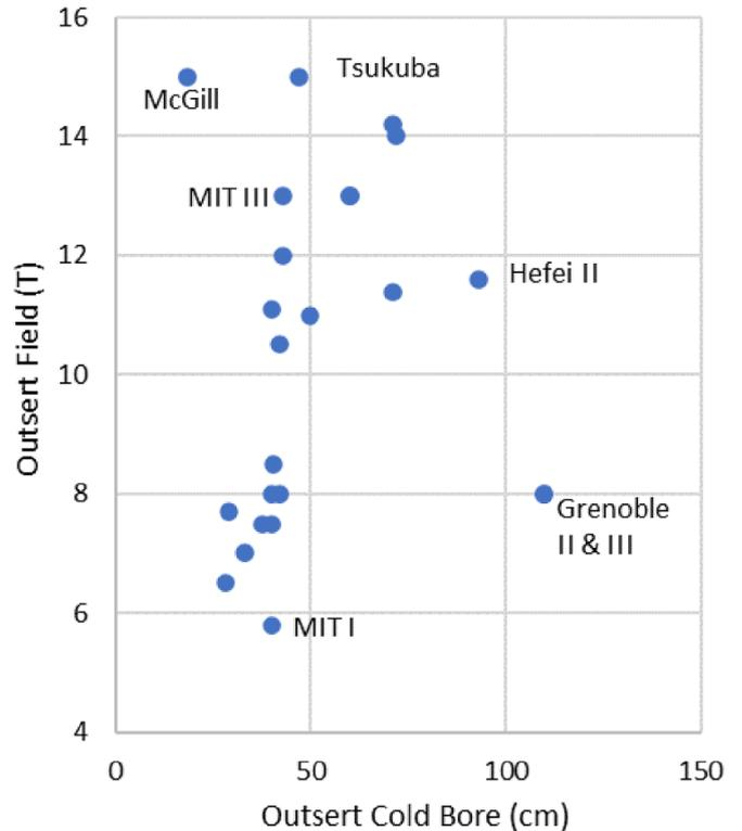
**Figure 6.** Field vs bore of hybrid outserts. The Grenoble II and III magnets have an extremely large bore for their fields.
