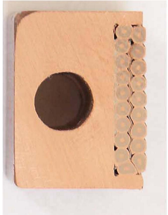
**Figure 9.** Rutherford Cable On Conduit conductor for the Grenoble III hybrid. The NbTi strands are. © (2011) IEEE. Reprinted, with permission, from [73].
