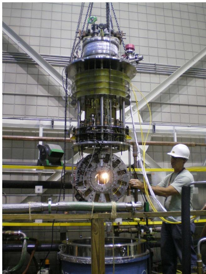
**Figure 7.** Preparing a Nb<sub>3</sub>Sn CICC for testing to high field and current while applying axial tension. (Photo Credit: MagLab Archives).
