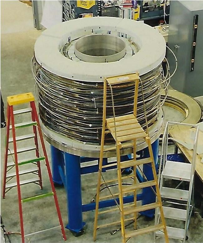
**Figure 5.** Photo of CICC coils of MagLab I after being assembled and prior to the helium vessel being closed. [Photo Credit: MagLab archives].
