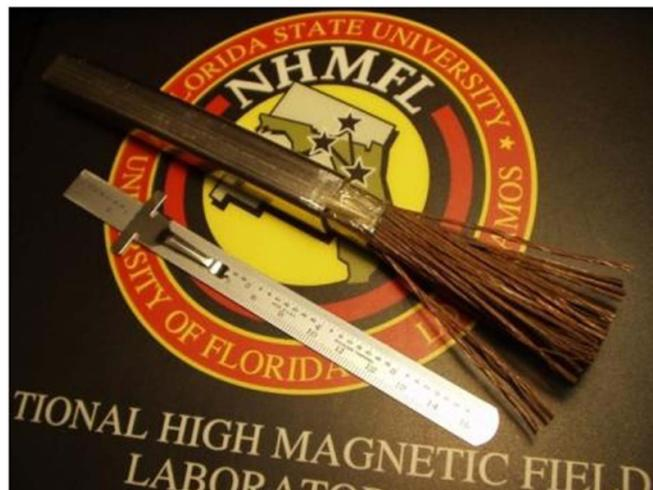
**Figure 4.** A piece of cable-in-conduit conductor (CICC) from the 45 T hybrid magnet in Tallahassee (MagLab I). This approach has now been incorporated into five different hybrids worldwide.
