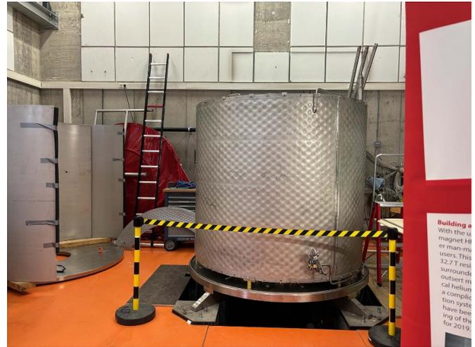
**Figure 11.** The cold mass of the Nijmegen III hybrid in 2024.
