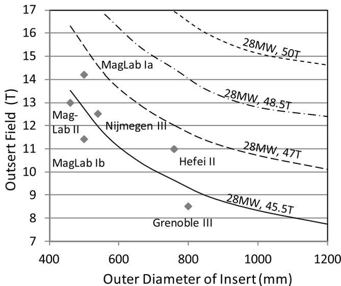
**Figure 12.** Field and space available for the resistive insert of several hybrid magnets worldwide along with projections of the field and bore size required for hybrid magnets extending to 50 T using 28 MW of power.
