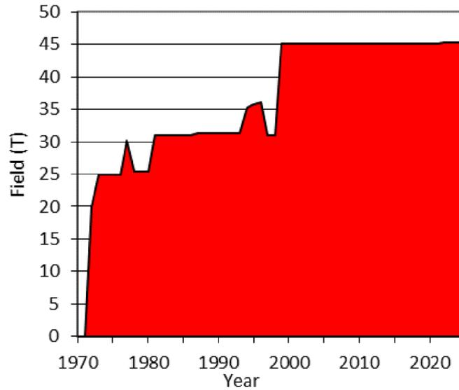
Figure 1. Fields available from hybrid magnets versus time.
