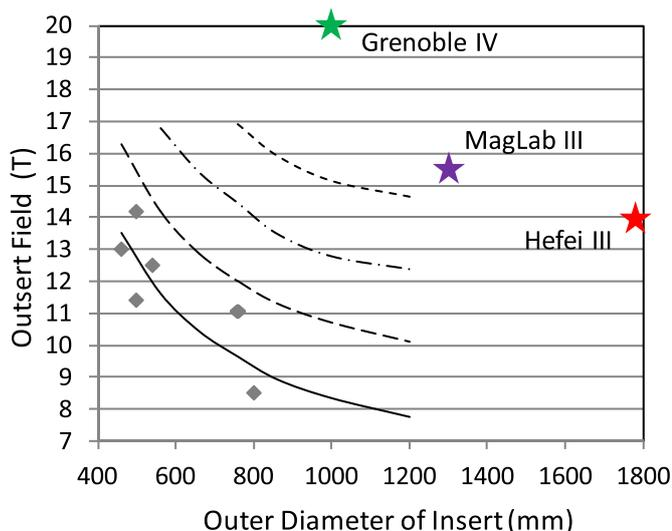
**Figure 13.** Field and bore of potential LTS coils of higher field hybrids being considered in Tallahassee, Grenoble, and Hefei compared with the largest existing hybrid outserts today.
