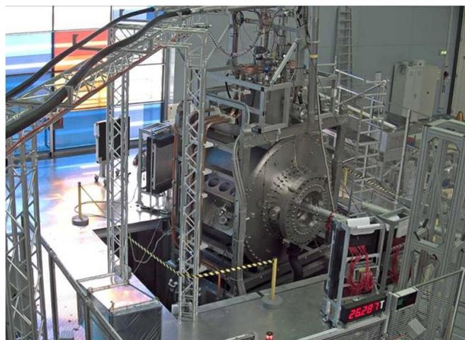
**Figure 8.** The 26 T hybrid magnet from the MagLab operating at the Helmholtz Zentrum Berlin in 2015. The neutron beamline enters the magnet from the right. Some neutron detectors are visible on the left of the magnet. (Photo Credit: MagLab Archives).
