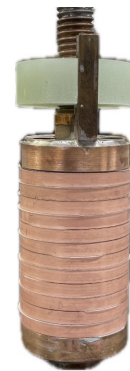
Fig. 1. Left : Basic parameters of LBC6 compared to LBC1—4. Conductor orientation can affect SCS via widthwise J_c gradients and ab -plane tilts, meaning that one winding orientation corresponds to lower SCS. Right : LBC6 before instrumentation.
